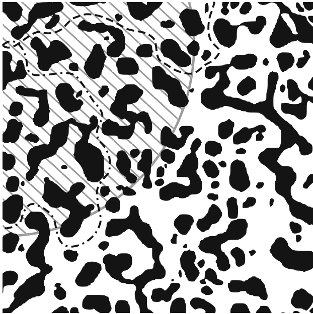
Fig. 1 Schematic illustration from Ref. [88] of the local percolation criterion (21). The grey hatched circle centered at \mathbf{p}_0 is the forbidden ball \mathbb{B}(\mathbf{p}_0, |\mathbf{r} - \mathbf{p}_0|) . Two paths are shown that start at \mathbf{p}_0 on the left boundary. The dashed path is percolating according to the percolation criterion (21), because it ends outside the forbidden ball. The dash-dotted path is not percolating, because it ends inside the forbidden ball
