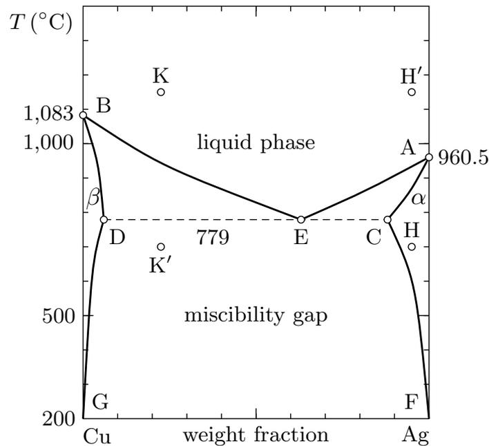
In the range of values given, this system has precisely three different phases. One liquid phase and two different solid solution phases. The  $\beta$ -solid solution phase is in the area BDG to the left and the  $\alpha$ -solid solution phase is in the area ACF to the right. The point E in the diagram is the eutectic point at which the liquid and both solid solution phases coexist.
