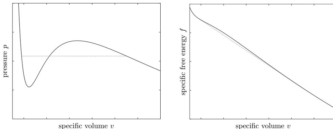
**Figure 2:** A typical isotherm for  $T < T_*$ : Left: in the  $(p, v)$  plane, Right: in the  $(f, v)$  plane. In both cases, the solid line represents the values obtained by directly using (1). The dotted line shows the Maxwell construction.
