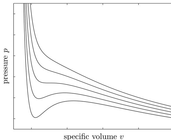
**Figure 1:** Isotherms of the van der Waals gases for five different temperatures. The center isotherm is the critical one. The constants are  $a = 0.01$  and  $b = 1$ .
